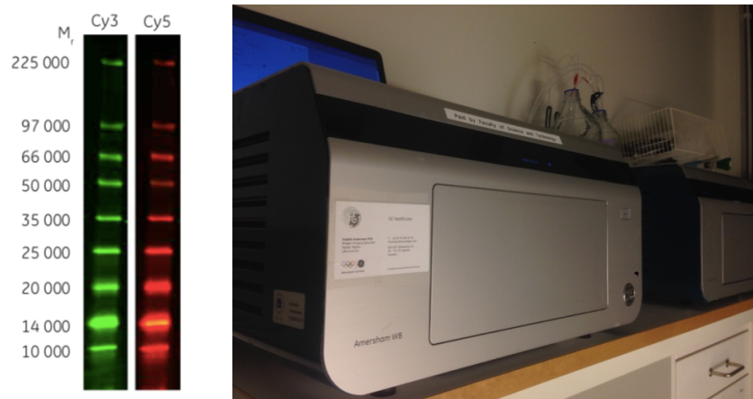
Figure 3: Left, molecular weight ladder used for the WB. Right, Amersham® electrophoresis & scan unit.
