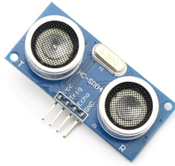
Figure 1.2. HC-SR04 ultrasound sensor has a transmitter (T) and a receiver (R) [3]
