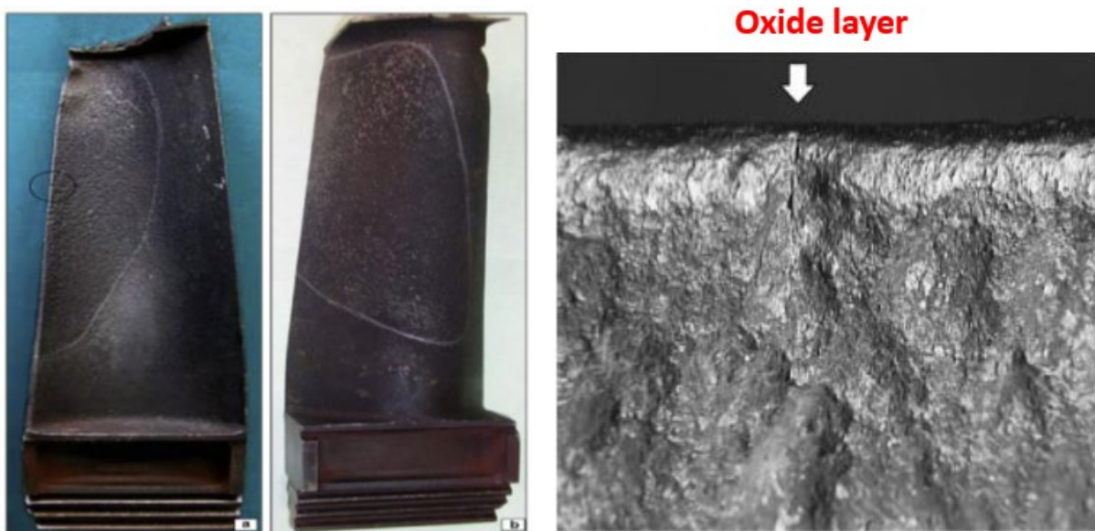
Figure 1.2: A corroded gas turbine blade of an aircraft (left) and formed oxide layer (right).
