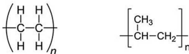
Figure 14. Molecule structure of polyethylene (left) & polypropylene (right). [37]
