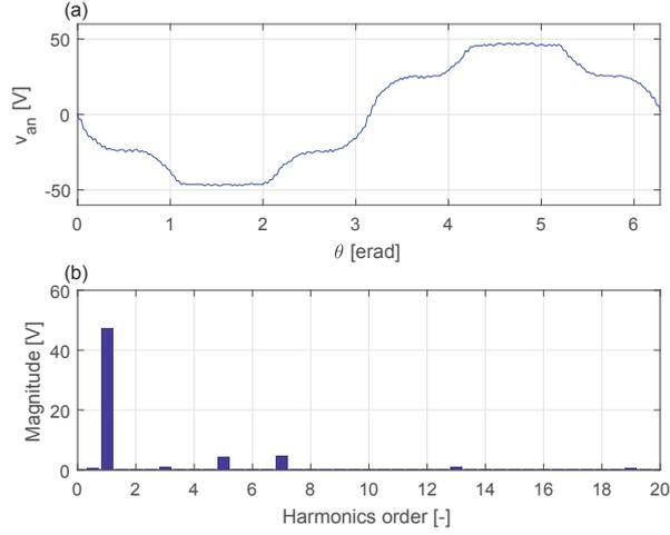
Figure 2: Harmonic analysis in stator winding of FSCW PMSM; (a) phase voltage, (b) harmonic order.
