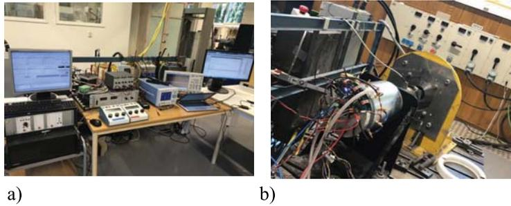
Figure 6: Experimental setup (a) power supplies and control set up, (b) FSCW PMSM connected to one submodule.
