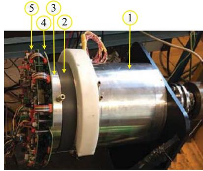
Figure 5: The proposed IMED topology; 1: electric motor (FSCW PMSM), 2: current sensors enclosure, 3: water cooling plates, 4: power boards, 5: control boards.
