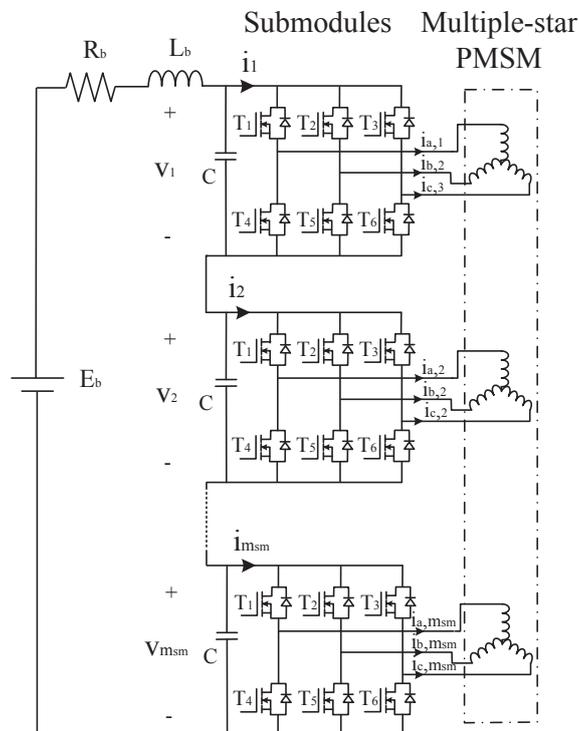
Figure 1: Schematic diagram of the proposed IMED topology (integration between SPB converter and FSCW PMSM).
