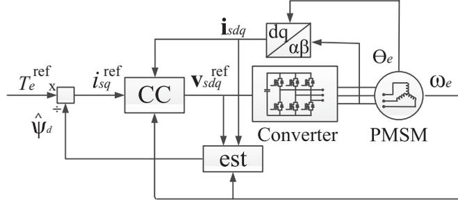
Figure 3: Schematic diagram of the current control (CC) and estimation (est) system.
