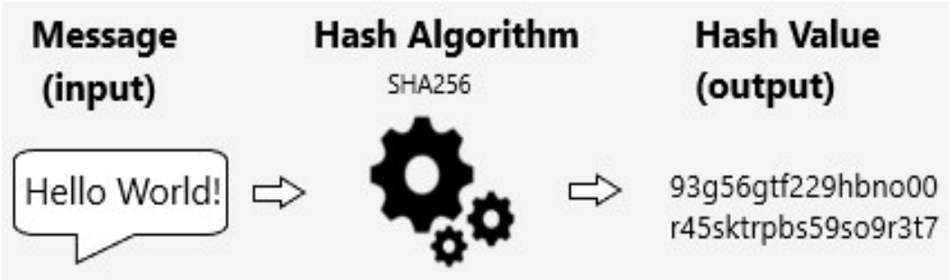
Image 5: By using a hash algorithm, a message or any type of information or value is translated to a fixed length of letters and numbers.
