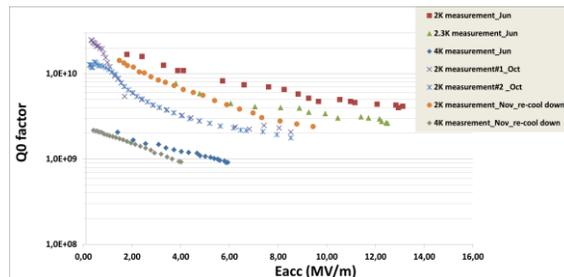
Figure 2:  $Q_0$  factor vs. Eacc curve of Germaine at FREIA.
