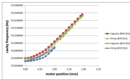
Figure 8: Tuning performance of double spoke cavity's CTS.
