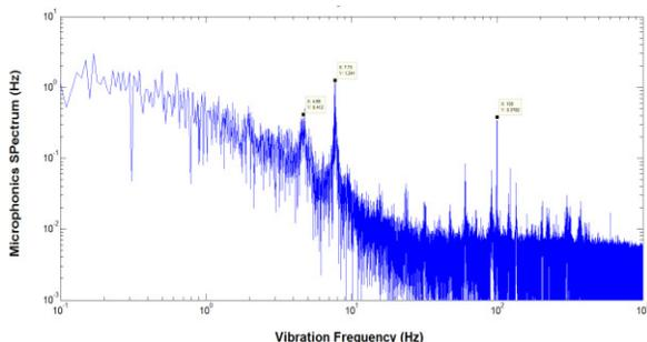
Figure 7: Microphonics measurement at 2K @31mbar. There are 3 main resonances: 4.6, 7.7 and 100 Hz.
