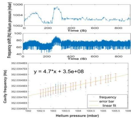
Figure 4: Pressure sensitivity of Germaine, where top and middle graphs are the helium fluctuation and frequency shift, respectively.
