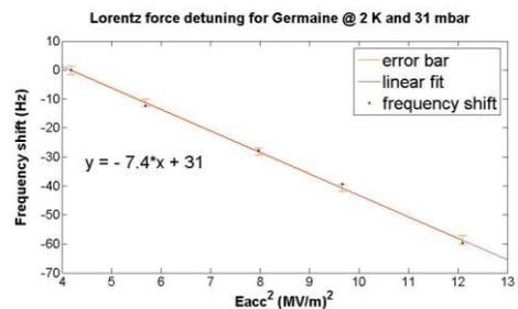
Figure 5: static Lorentz detuning curve of Germaine after pick-up coupler repaired.
