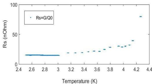
Figure 3: Rs vs. T measurement of Germaine at a fixed gradient.
