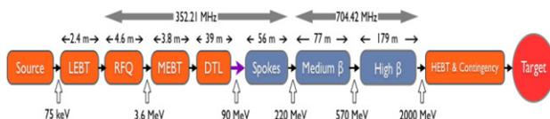
Figure 1: The layout of ESS accelerator.
