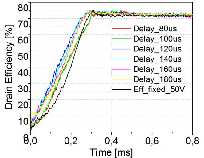
The temporal drain efficiency is presented at Fig.1. During the filling time, the drain efficiency at low power levels is improved by 100% as compared to the case when using a constant drain voltage. In the presented implementation, the overall wall plug efficiency is improved by 24%, **see cite your paper 1**.
