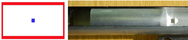
Figure 1: Simulated (a) and real (b) aluminum sample holder tubes.
