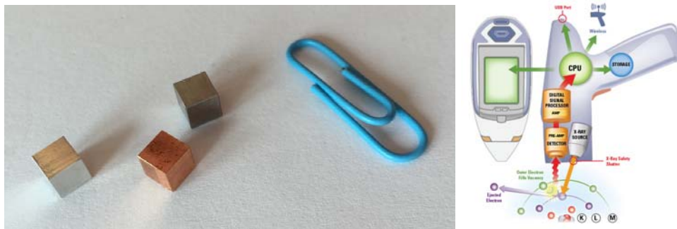
Figure 3: Metal samples (aluminium, stainless steel and copper) and handheld XRF device.
