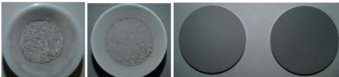
Figure 4: Grained concrete and pressed concrete pellets for XRF analysis.
