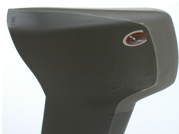
Figure 4-2. Close-up view of a BERP rotor blade tip
