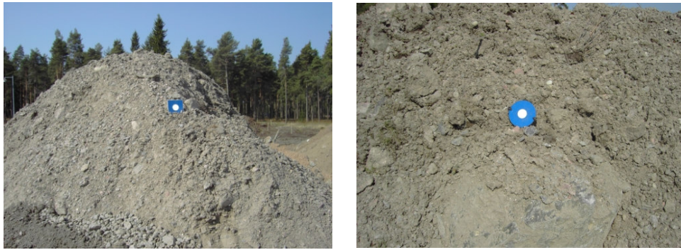
Figure 8: on the left: planar target; on the right: half sphere ( each on the pile )
