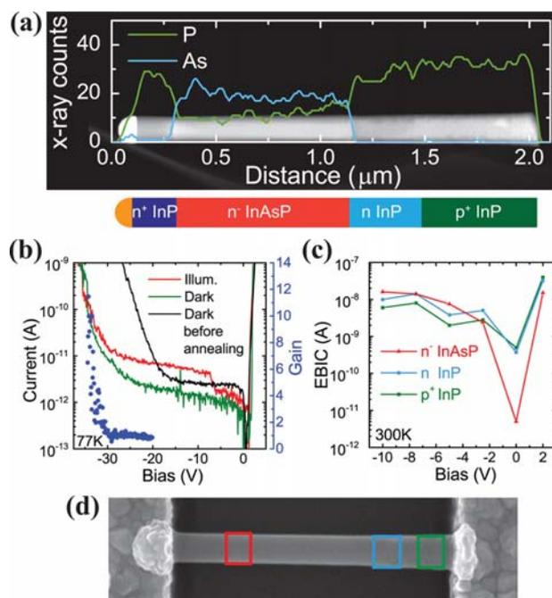
**Figure 2.** (a) EDX line scans superimposed on a TEM image, along with a schematic of an InP/InAsP NW SAM APD (sample B). (b)  $I$ – $V$  characteristics and gain at 77 K of an InP/InAsP NW SAM APD in the dark, before and after annealing, and under selective illumination of the InAsP absorption region. (c) Electron-beam-induced current (EBIC) versus bias characteristics corresponding to e-beam excitation in (d). (d) Spatially resolved e-beam excitation map over the length of the NW.
