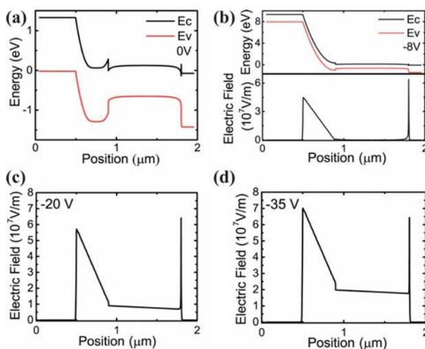
**Figure 3.** Characteristics of the InAsP SAM APD at 300 K: (a) Band profile at 0 V. (b) Band profile at punch-through ( $-8$  V, upper panel) and corresponding electric field distribution (lower panel). (c) Electric field distribution at  $-20$  V. (d) Electric field distributions at the approximate breakdown voltage of  $-35$  V.
