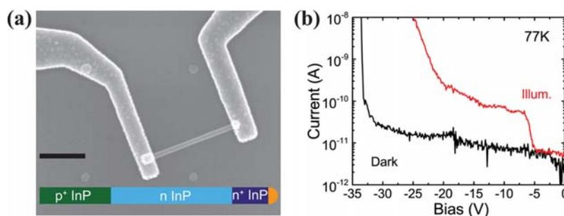
**Figure 1.** (a) SEM image of a laterally contacted p<sup>+</sup>-n-n<sup>+</sup> InP NW device along with the schematics. The scale bar is 1 μm. (b) Avalanche breakdown characteristics of a corresponding device at 77 K under darkness and illumination, respectively.
