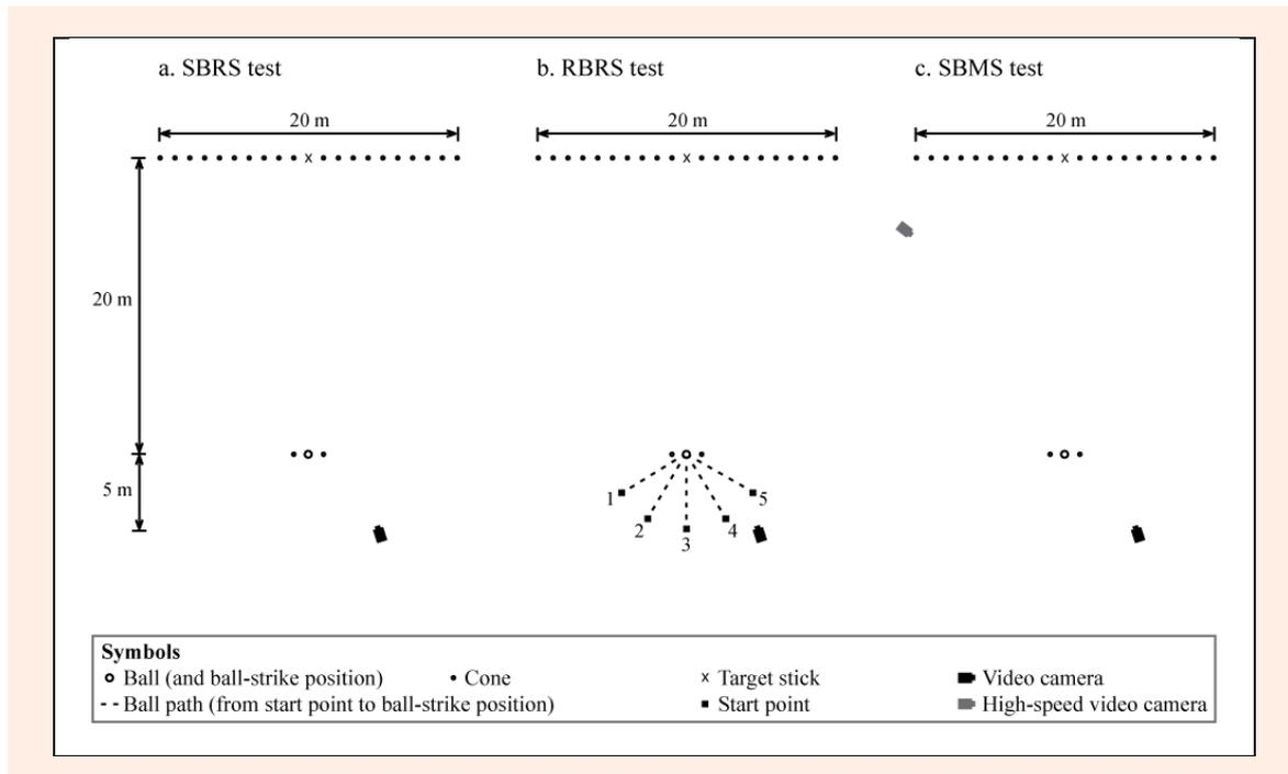
**Figure 1.** The arrangement of the three side foot-kick tests. a) SBRS test with freely chosen approach angle, stationary ball, and match-relevant ball speed; b) RBRS test with fixed approach angle ( $0^\circ$ ,  $30^\circ$ , and  $60^\circ$ ), moving ball, and match-relevant ball speed; c) SBMS test with freely chosen approach angle, stationary ball, and maximal ball speed while maintaining a high accuracy.
