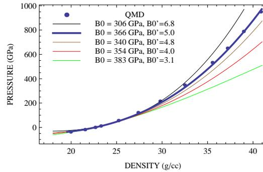
**Figure 2.** The  $T=0$  Ir EOS from VASP compared to the experimental and theoretical 300 K Birch-Murnaghan EOSs.
