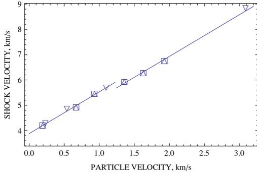
**Figure 1.** Shock velocity,  $U_s$ , vs. particle velocity,  $U_p$ , along the principal Hugoniot in Ir; data from [7]. A solid-solid phase transition occurs at  $1.10 < U_p < 1.36$  km/s.
