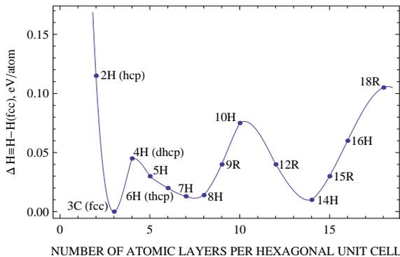
**Figure 3.** Differences between the  $T=0$  enthalpies of hex structures of Ir and that of *fcc*-Ir as a function of the number of atomic layers per unit hex cell, at a fixed unit cell volume.
