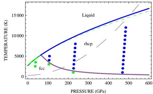
**Figure 4.** Phase diagram of Ir obtained from the Z methodology: *fcc*-Ir melting curve (green line), liquid Ir solidified into solid fcc (green bullets), *9R*-Ir melting curve (blue line), liquid Ir solidified into solid rhcp (blue bullets), and the (tentative) fcc-rhcp solid-solid phase boundary (violet).
