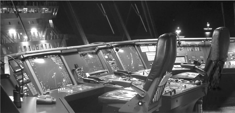
*Figure 6: A modern centre console on a high-speed ferry bridge.*
