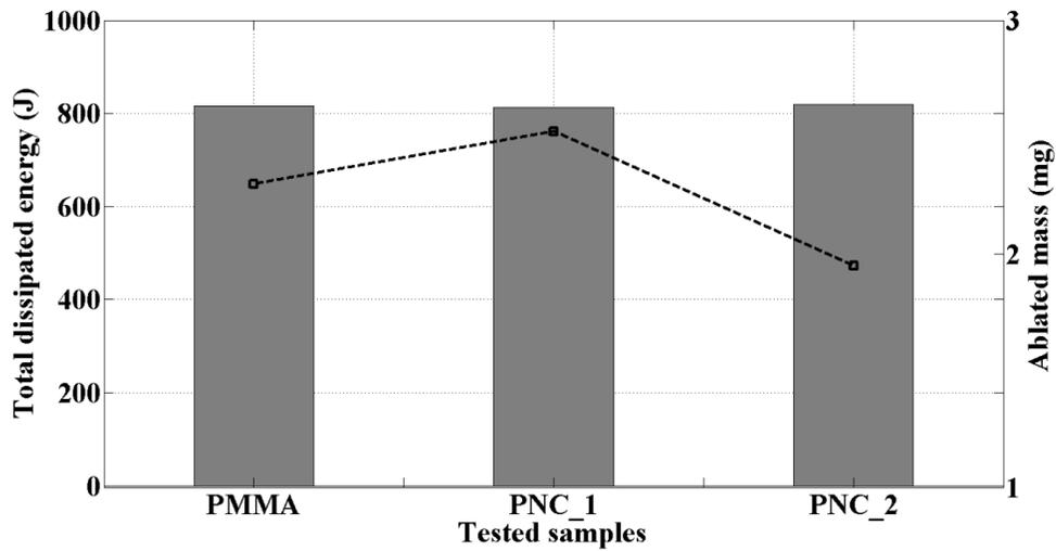
Figure 4. Total dissipated energy (bar plot) and recorded ablated mass (dashed line) using the tested samples i.e. PMMA and PNCs.
