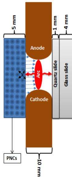
Figure 2. Illustration of the PNCs and experimental test-setup used for the tests with electrical arcs.
