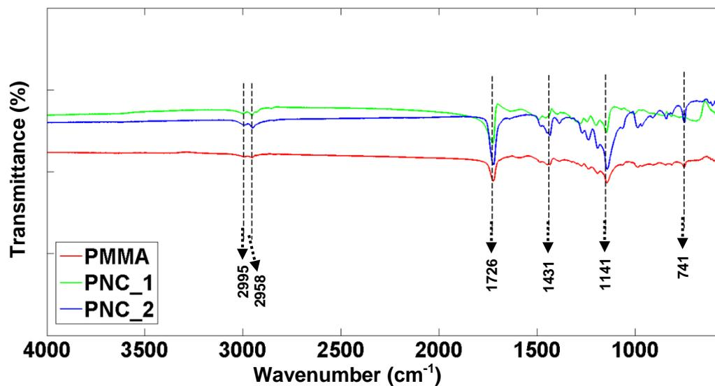
Figure 5. FT-IR spectrum of the deposited outgassed chemical species on the PMMA and PNCs.
