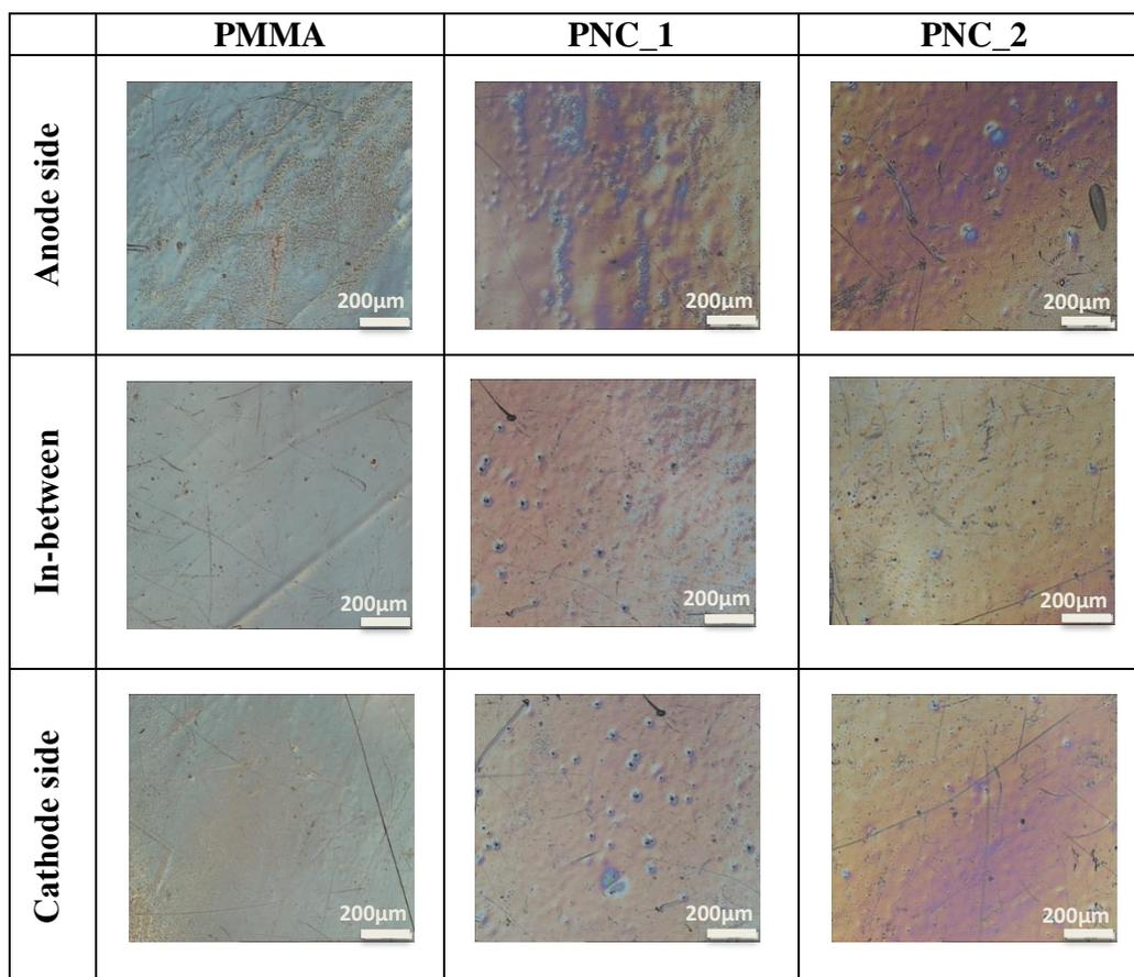
Figure 6. Optical micrographs of the outgassed PMMA and PNCs after three discharges in different locations.
