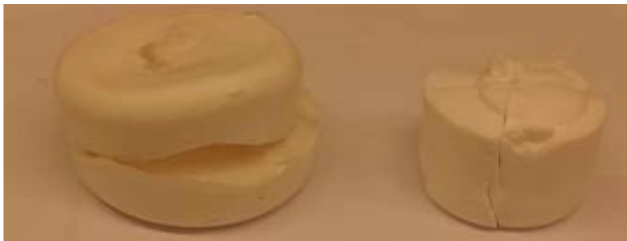
Figure 3a. Foam material from freeze-dried NFC: The left foam material is NFC from TEMPO method. The right foam material is NFC from formic acid method.
