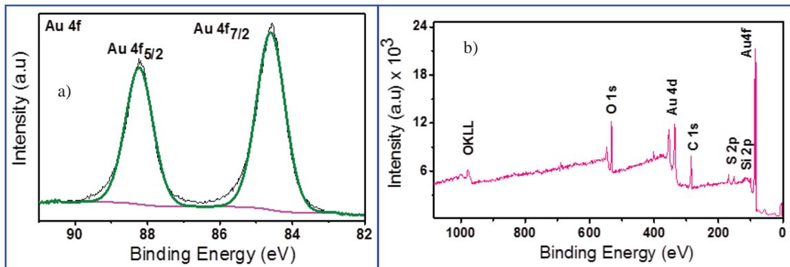
**Fig. 3.** XPS spectra of: a) Au4f core level splitting; b) AuNPs capped with 4-methoxy-  $\alpha$ -toluenethiol.
