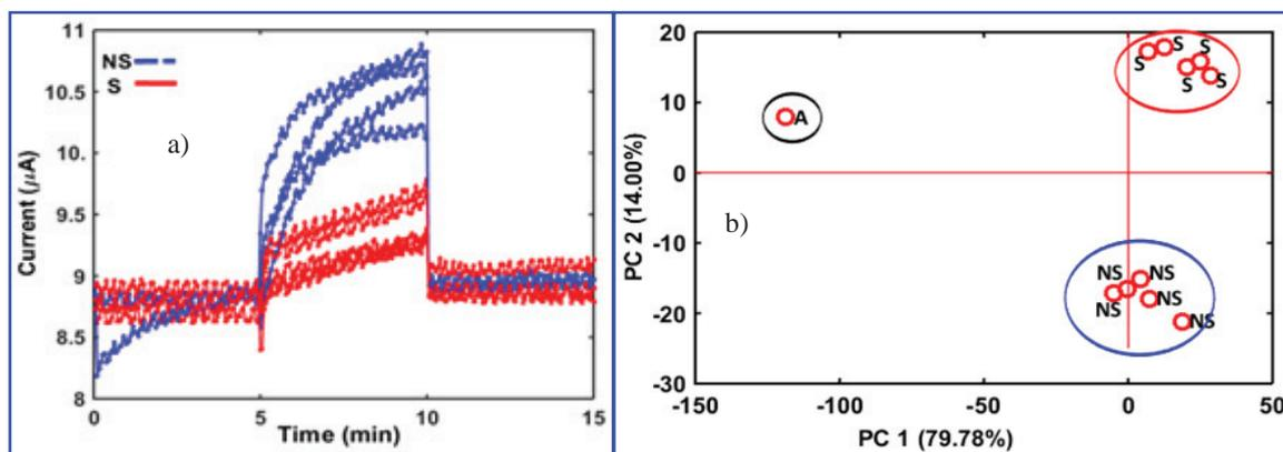
Fig.4. a) Responses of the 4-methoxy- $\alpha$ -toluenethiol capped AuNPs sensor to the exhaled breath of the 5 smokers and 5 non-smokers volunteers; b) PCA plot showing excellent discrimination of exhaled breath samples of smokers, non-smokers, and ambient air.
