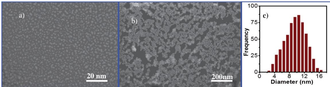
**Fig. 2.** SEM images of: a) dispersed AuNPs; b) AuNPs functionalized with 4-methoxy-  $\alpha$ -toluenethiol; c) AuNPs crystallite size distribution
