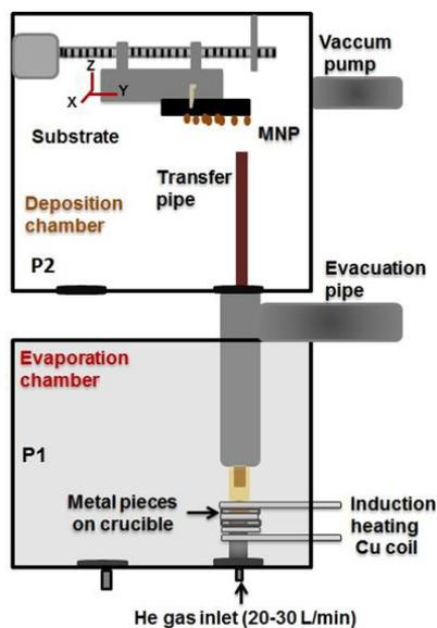
Fig. 1. Advanced Gas Deposition (AGD) technique adapted for AuNPs fabrication and deposition.
