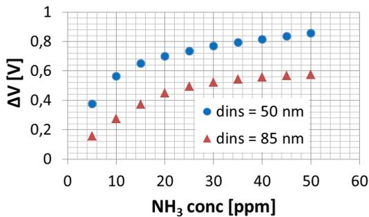
Fig. 2 displays the increase in sensor response (sensor voltage signal change,  $\Delta V$ ) upon a decrease in gate insulator thickness (dins), as exemplified by the exposure of the sensor devices to different concentrations of ammonia
