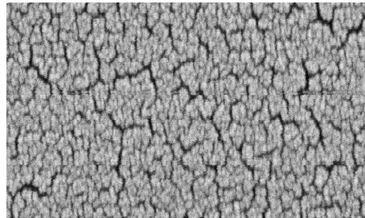
Fig. 3 displays an example of a nanostructured thin-film of Ir applied as gate contact in a SiC-FET gas sensor device, in this particular example deposited by DC magnetron sputtering
