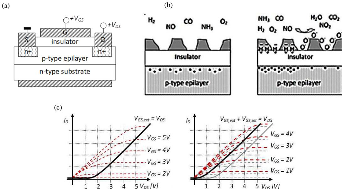
Fig. 1 displays in (a) the basic cross-sectional design of a field effect transistor based gas sensor and in (b) and (c) the change in the number of mobile charge carriers in the top part of the semiconductor upon gas exposure and the resulting change in I/V characteristics, respectively.
