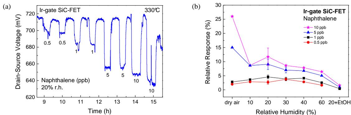
Fig 4 (a) Sensor response to ultra-low concentrations of naphthalene from 0.5 to 10 ppb; (b) Relative response to naphthalene as a function of the relative humidity. The figure shows also the effect of 0.5 ppm ethanol (EtOH), introduced as interfering gas, to the sensor response.
