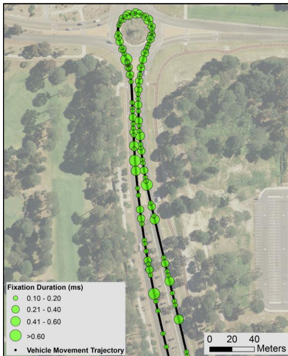
Figure 9. The spatial distribution of eye fixation behaviour at a roundabout U-turn and straight road driving from one driver.
