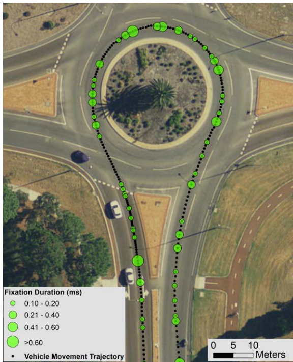
Figure 2. The spatial distribution of eye fixation behaviour at roundabout U-turn from driver A
