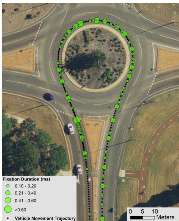
Figure 3. The spatial distribution of eye fixation behaviour at roundabout U-turn from driver B
