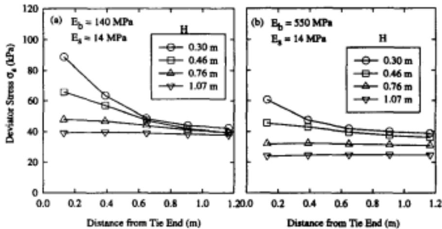
Figure 15. Deviator stress at subgrade surface for different thickness and resilient modulus of the trackbed layer. Figure a) Trackbed resilient modulus = 140 MPa, b) trackbed resilient modulus 550 MPa (Li and Selig, 1998)
