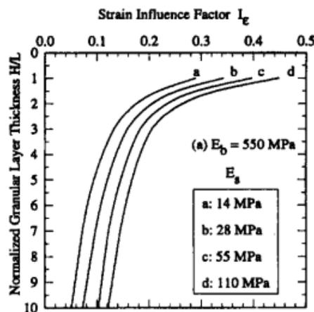
Figure 9. Example of design chart, the soil type is selected from Table 2. (Li and Selig, 1998)
