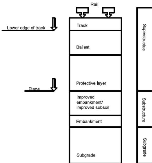
Figure 25. General ballasted track solution
