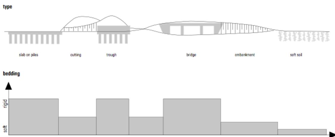
Figure 6. Different earthwork and the variation in stiffness (SSF Ingenieure, 2010)
