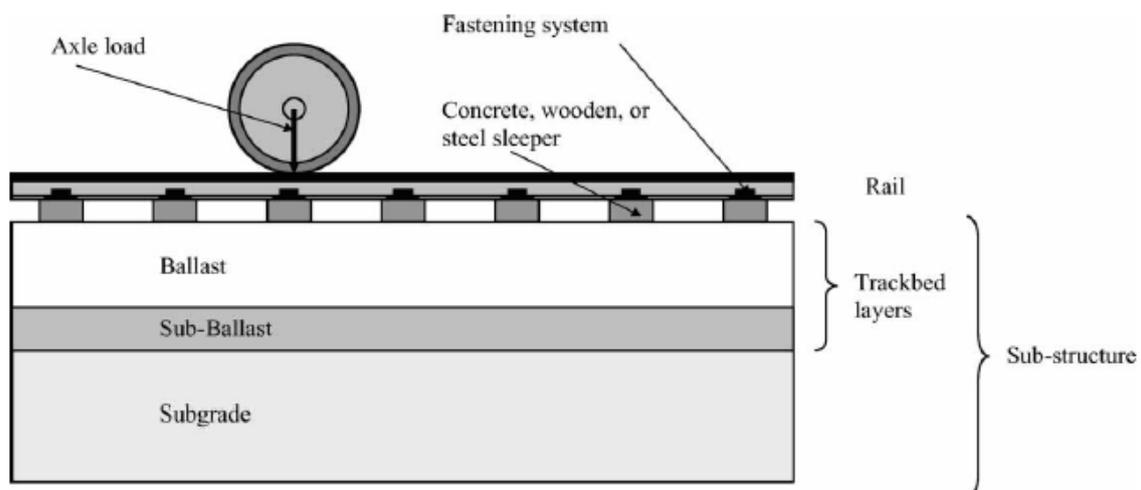
Figure 2. Simplified components of a typical ballasted track (Burrow, Bowness, and Ghataora, 2007).
