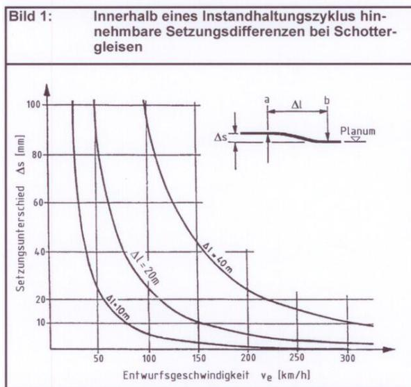
Figure 20. Requirements for the differential settlements. On the x-axis shows the design speed [km/h] and on the y-axis shows acceptable differential settlements [mm].
