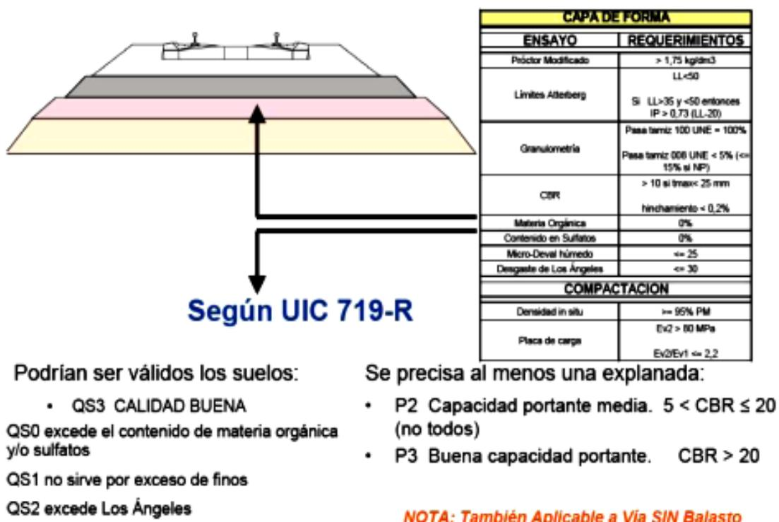
Figure 7. Formation layer according to UIC 719 –R (Smekal, 2012)
