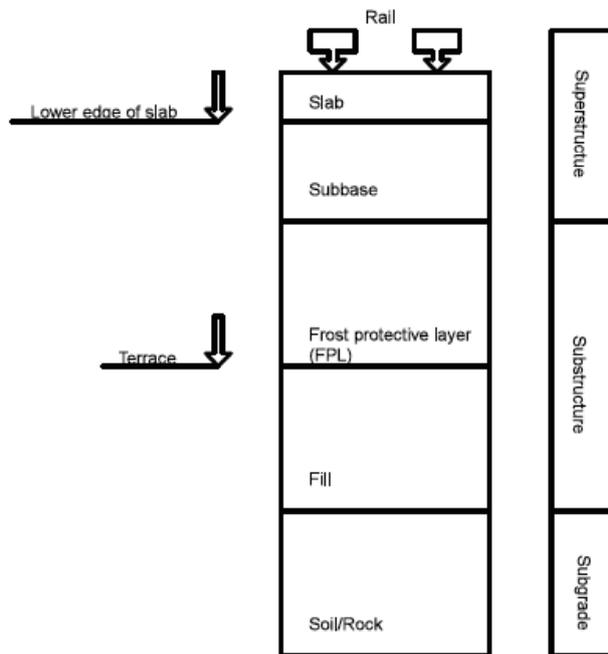
Figure 24. Principal definition of ballastless embankment, with superstructure and substructure.
