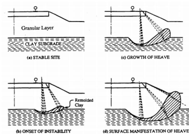
Figure 2. Progressive shear deformation (Selig and Waters, 1994; Li and Selig, 1995)
