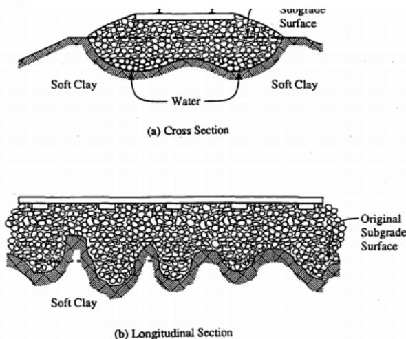
Figure 5. Excessive plastic deformation (Selig and Waters, 1994; Li and Selig, 1995)
