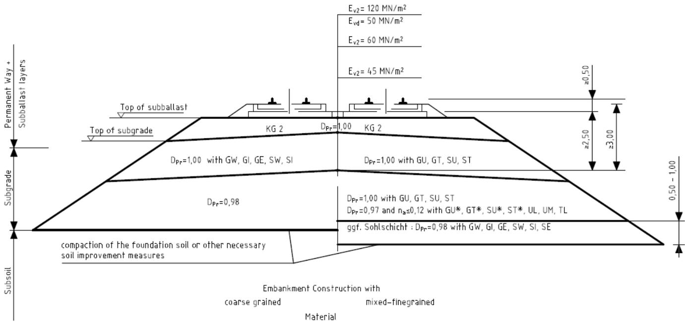
Figure 21. General German design principle for a ballastless high-speed embankment (Swedish Transport Administration, 2012)
