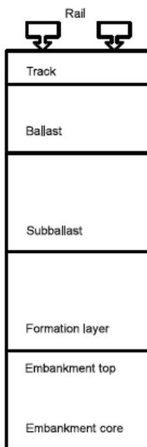
Figure 29. Definition according to UIC 719-R
