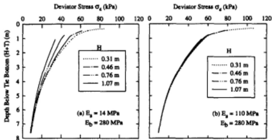
Figure 16. Deviator stress at subgrade surface for a) soft subgrade, 14MPa and b) stiff subgrade, 110 MPa for varying thickness of the trackbed layer (Li and Selig, 1998)
