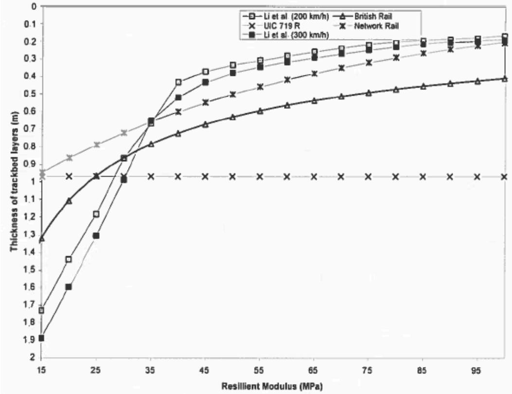
Figure 14. Variation in designed trackbed thickness, depending on design method and the resilient modulus in the subgrade (Peter, Burrow, Ghataora, and Evdorides, 2011).
