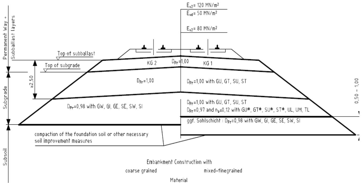
Figure 22. General German design principle for a ballasted high-speed embankment (Swedish Transport Administration, 2012)
