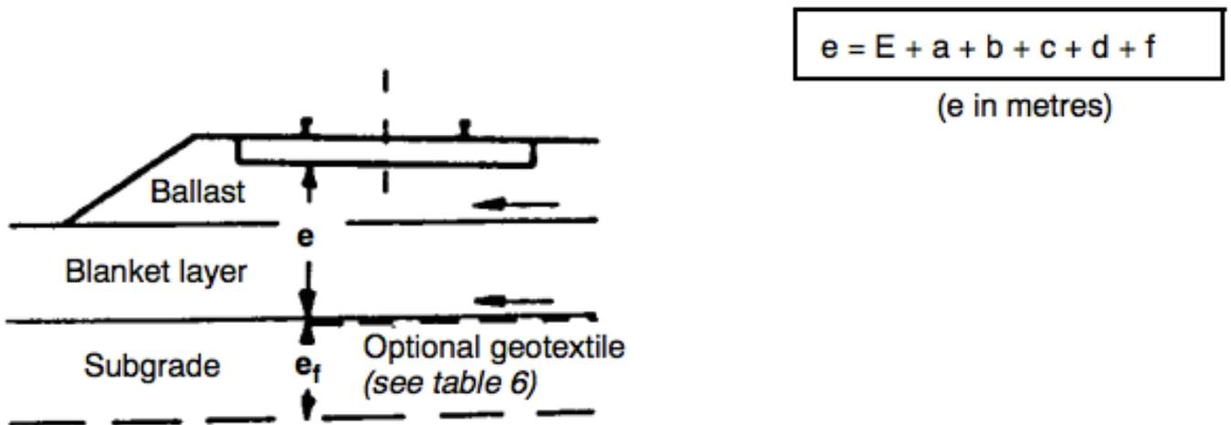
Figure 12. Minimum thickness of trackbed layer,  $e$ [m] (UIC, 2008).
