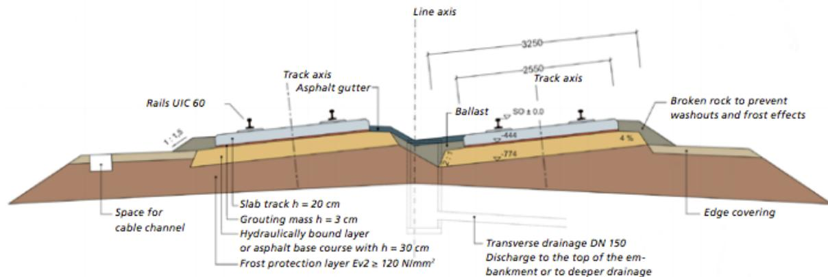
Figure 4. Typical cross-section for a Bögl slab track on an earth structure (Max Bögl).
