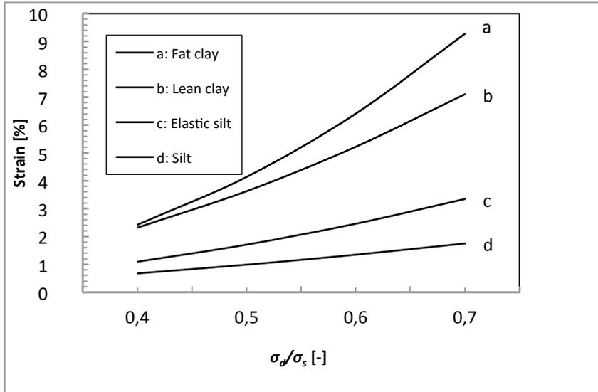
Figure 7. Cumulative plastic strain variation, depending on ratio of deviator stress and compression strength
