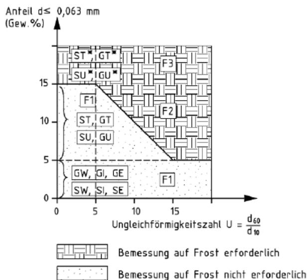
Figure 27. Classification of frost susceptibility as a function of percentage fine-grain in the material, d, and coefficient of uniformity, U. The dotted area shows the materials where frost dimensioning is not required and the hatched area shows the material where frost dimensioning is required. (DB Netze AG, 2014)
