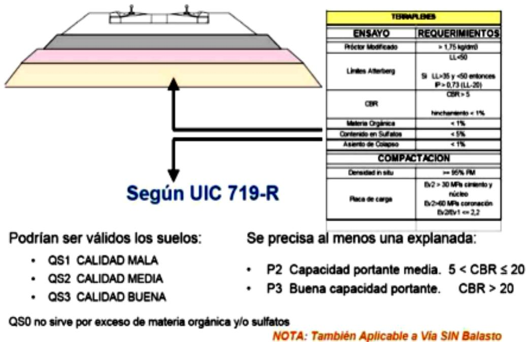
Figure 6. Embankment layer according to UIC 719 –R (Smekal, 2012)
