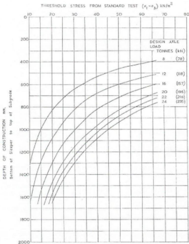
Figure 13. Design chart used to determine the stress threshold value, from (Heath et al., 1972) .
