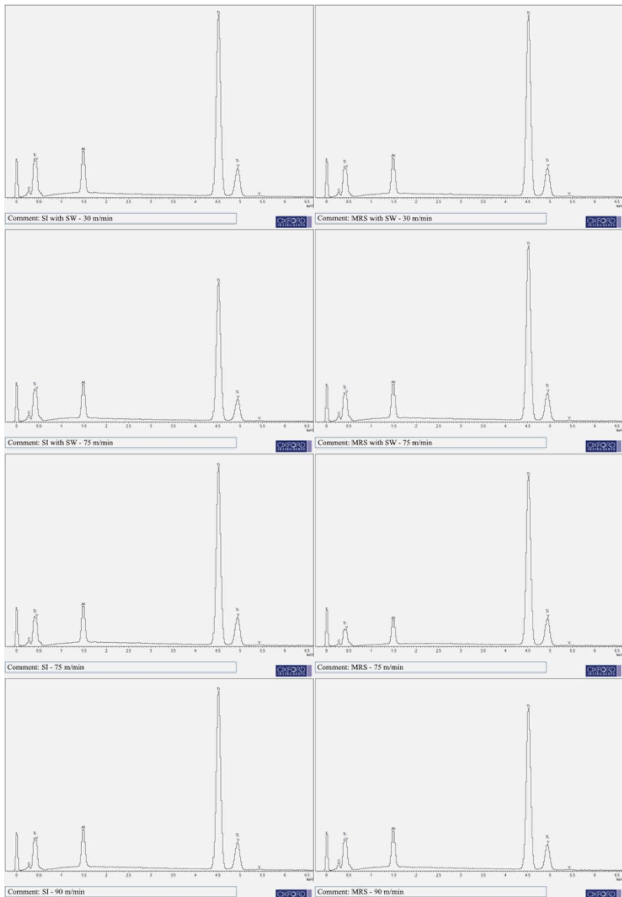
**Figure H1.** EDS analysis of the back side of the chips eight chips at different cutting conditions.
