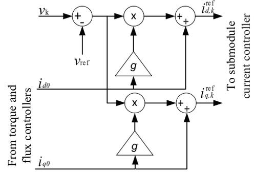
Fig. 2. Block diagram of the balancing controller.
