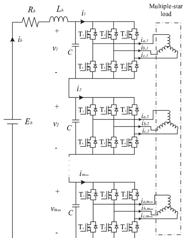
Fig. 1. The SPB converter topology with  $m_{sm}$  submodules.
