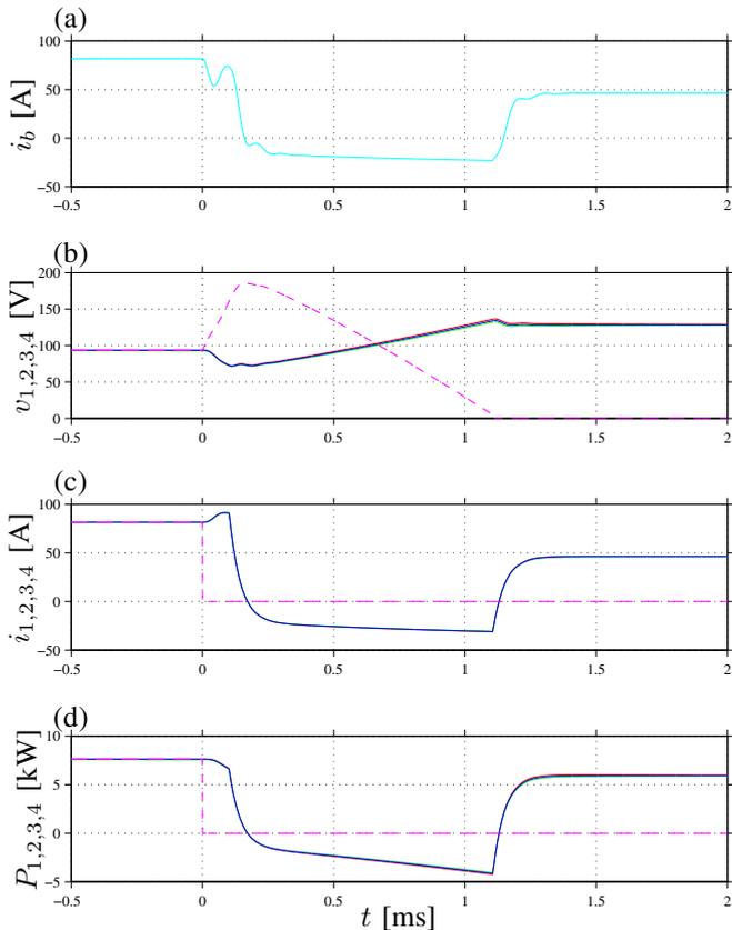
Fig. 5. A short-circuit fault on  $T_1$  of submodule 4: (a) Current drawn from the voltage source (e.g., battery). (b) Capacitor voltage for the  $k$ th submodule; red, green, blue, and magenta respectively for  $k = 1, 2, 3, 4$ . (c) Current into the  $k$ th submodule; red, green, blue, and magenta respectively for  $k = 1, 2, 3, 4$ . (d) Power into the  $k$ th set of windings; red, green, blue, and magenta respectively for  $k = 1, 2, 3, 4$ .
