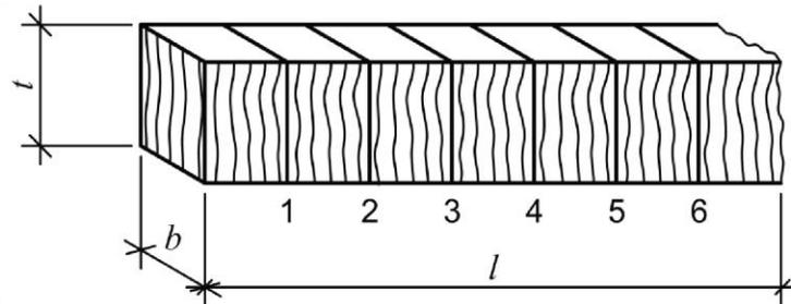
**Fig. 1.** Tested sample of glulam (adapted from SS-EN 14080 (2013) (Fig. D. 2))
