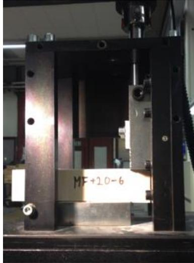
Fig. 2. Shear test machine and test specimen
