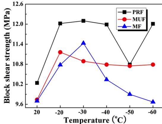
**Fig. 3.** Bondline block shear strength of Norway spruce glulam joints bonded with three specified adhesives at various temperatures
