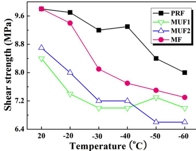
**Fig. 4.** Bondline shear strength (according to EN 302-1) of Norway spruce wood joints bonded with three specified adhesives at different temperatures (adapted from Wang *et al.* 2015)
