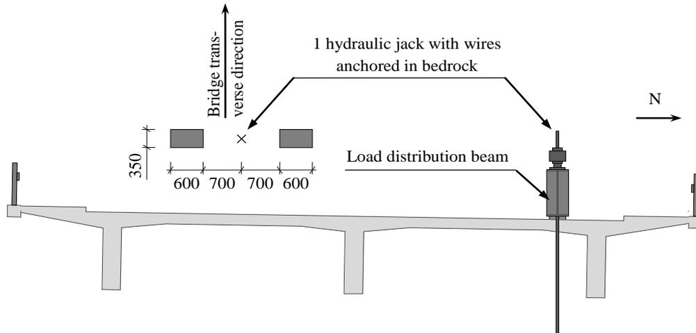
Figure 1: Arrangement for loading the bridge deck slab.
