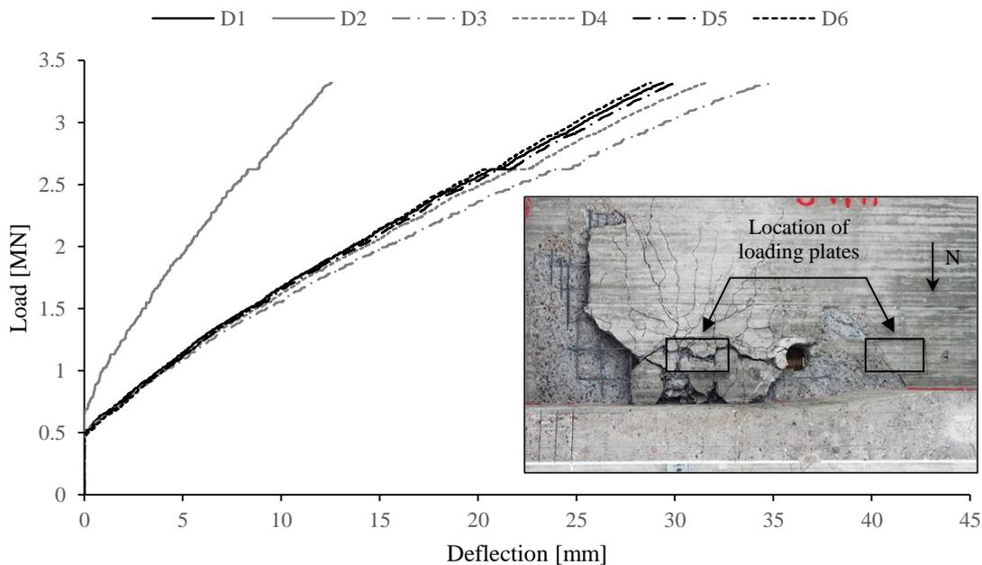
Figure 2. Measured load-deformation curves and photograph of punching failure (2014-07-01).
