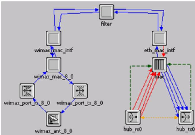
Figure 5: Node model for the WIMAX BS.
