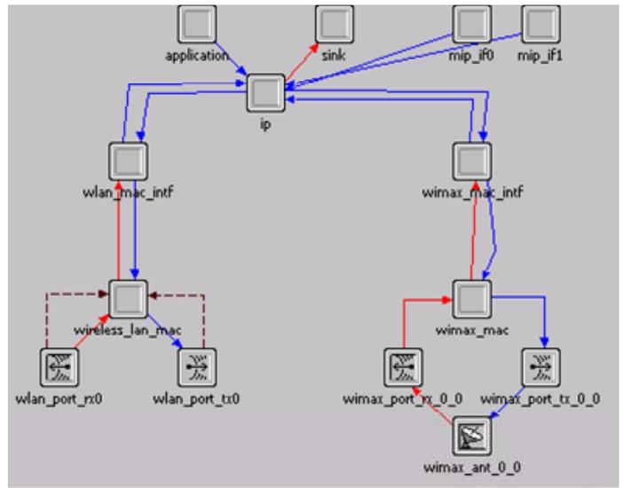
Figure 3: Node model for the mobile node.
