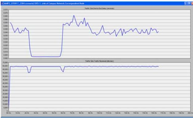
**Figure 10. End-to-end delay for payload traffic and received bandwidth at correspondent node.**
