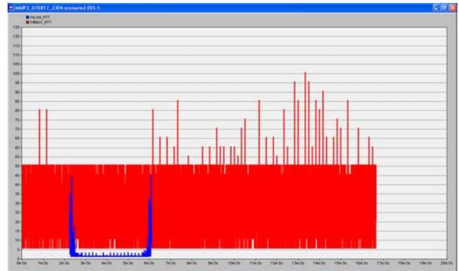
Figure 7: Round-trip delays in MIP BU/Back messages (WLAN/WIMAX).
