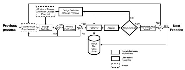
Figure 1. Proposed approach process flowchart for KBE, CBR and manual activities. Arrows that describe start of iteration are in boldface.
