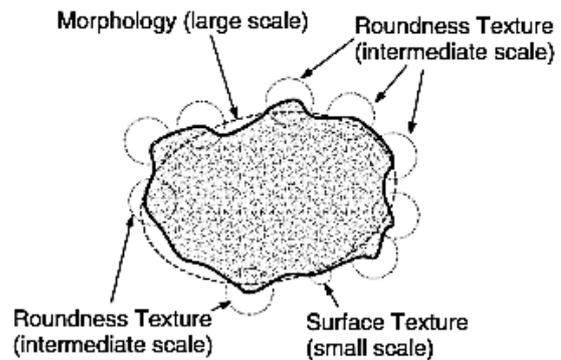
Figure 1. Scale descriptors of a grain (Mitchell & Soga, 2005).
